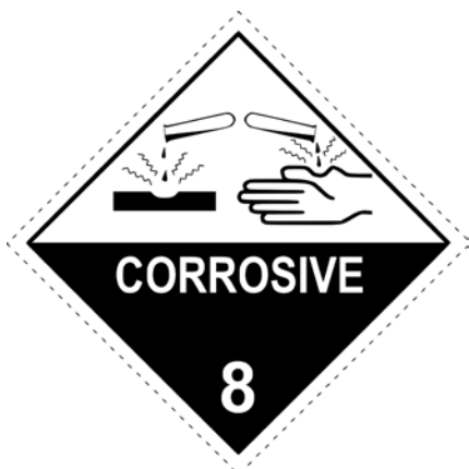
a) Marking for Class 8 dangerous goods according to the National Transport Commission (Australia).
