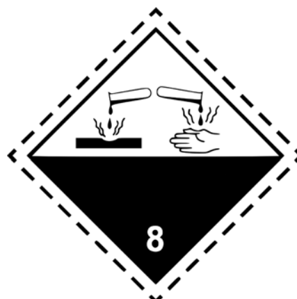
b) Marking for Class 8 dangerous goods according to the United Nations Economic Commission for Europe.
